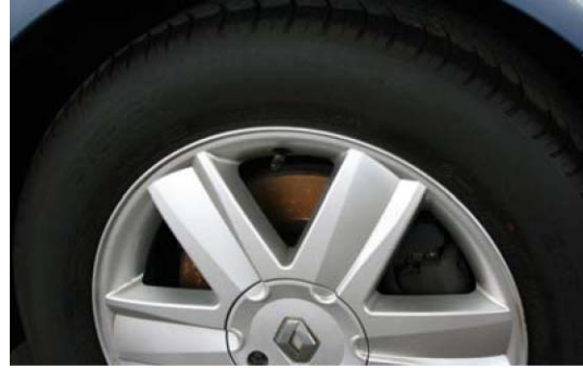
Sales Car suffering from corrosion (lot rot)
